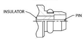
The MMCX, "miniature MCX", micro-miniature series of  $50\Omega$  connectors was developed in the 1990's for use with densely packed PCB layouts. They are about half the size of the SMB. Their locksnap coupling mechanism with non-slotted outer contact allows 360 degree rotation without loss of broadband performance and with low reflection from DC to 6 GHz. MMCX connectors conform to European
