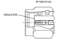
SMA Reverse polarity SMA connectors share the same performance characteristics of standard SMA's, but the pin and socket are reversed. If you are looking into the shell of the male connector and see a flush socket and dielectric rather than raised pin, you have a reverse polarity SMA male. A raised pin in an SMA female connector indicates reverse polarity SMA female.
