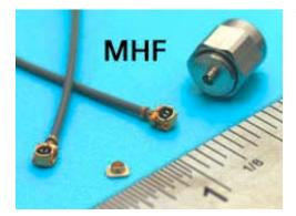
The MHF micro-coax connector is equivalent to the Hirose U.FL and Ipex series connectors found in many WiFi products. They are a low profile [2.5mm mating height] and support dual band 3-6 GHz applications.
