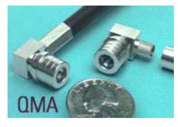
QMA connectors are quick disconnecting versions of SMA connectors; they snap on and off rather than mate by turning threads. QMA's couple in two seconds rather than twenty, but more importantly, they can be rotated 360 degrees after they are mated, optimizing the flexibility of installations and durability of jumpers. The QMA coupling mechanism creates a 360-degree butt joint that is maintained even with rotation, resulting in low RF leakage. Because QMA's are internally identical to SMA's,
