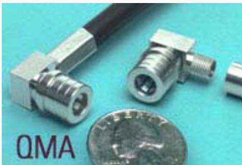
QMA connectors are quick disconnecting versions of SMA connectors; they snap on and off rather than mate by turning threads. QMA's couple in two seconds rather than twenty, but more importantly, they can be rotated 360 degrees after they are mated, optimizing the flexibility of installations and durability of jumpers. The QMA coupling mechanism creates a 360-degree butt joint that is maintained even with rotation, resulting in low RF leakage. Because QMA's are internally identical to SMA's,
