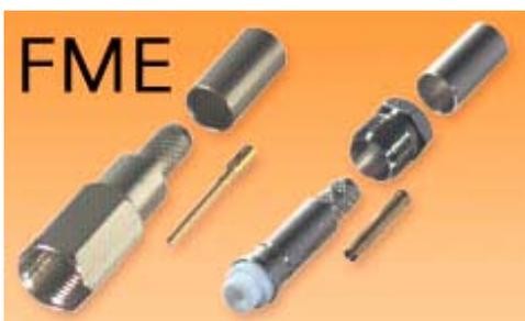
FME, or "Euro-Nipple", connectors originated in Europe and are used most prominently in antenna couplings. They have 50 ohm impedance and operate in the frequency range of DC to 200 MHz. They mate with M8XP .75 threads and the female has the distinctive "nipple" appearance.
