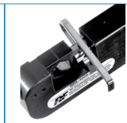
Lower die removal
